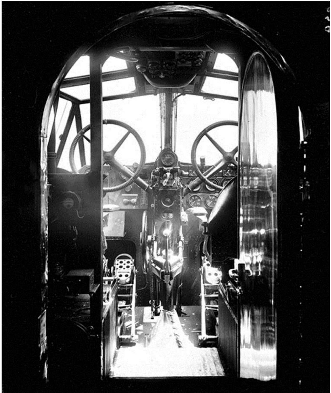
The cockpit of a Handley Page HP-42 airliner. London, 1931. No powered controls here.
