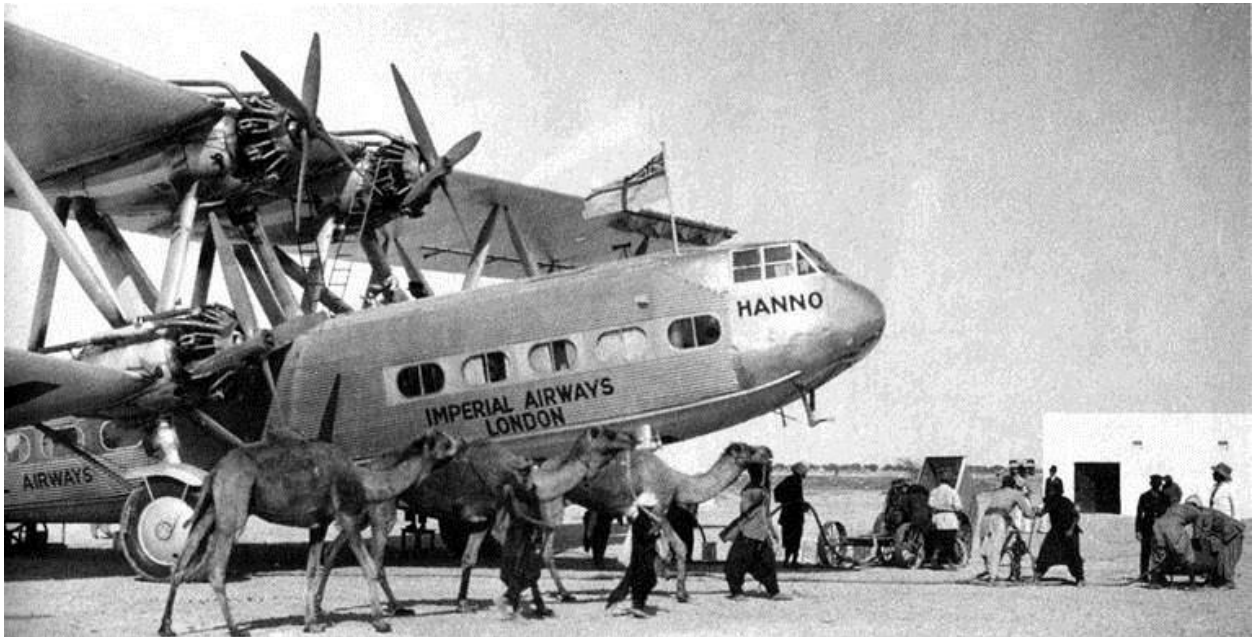
Imperial Airways at Cairo. 1932. Note the refueling equipment, including the ladders resting on the upper engines. Note, also, the modest terminal building.
